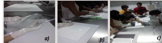
Fig.8. a) Unpacking the scintillator. b) y c) Lining to optimize capture of light from the signal.
